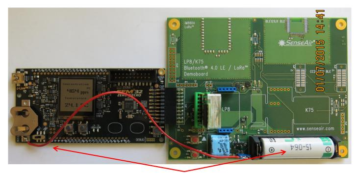
Battery on the Demoboard is used to power EFM32 Starter Kit. In turn Demoboard is supplied from the VMCU pin of the Starter Kit expansion connector.
