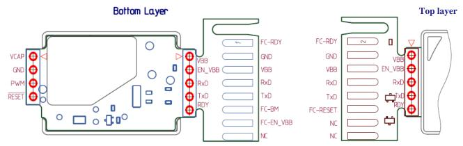
Note: VCAP and EN\_VBB are connected to VBB at Factory Connector (if sensor is supplied with Factor Connector).
