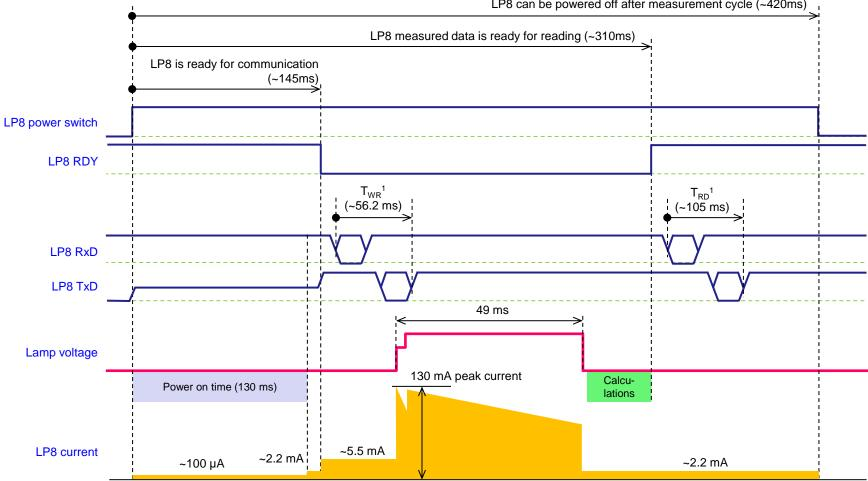
LP8 can be powered off after measurement cycle (~420ms)
