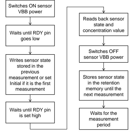
Measurement period of the sensor is determined by customer host system and may vary without degrading measurement accuracy. Minimum allowed measurement period is 16 seconds (below 16 seconds accuracy is not guaranteed).
